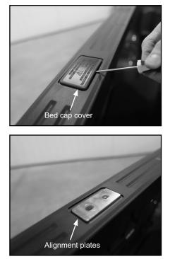
B. Place (3) alignment plates where bed cap covers were removed.
