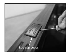
B. Place (3) alignment plates where bed cap covers were removed.
