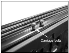
E. Secure with (2) flat washers and (2) nylock flange nuts, fully tighten.
