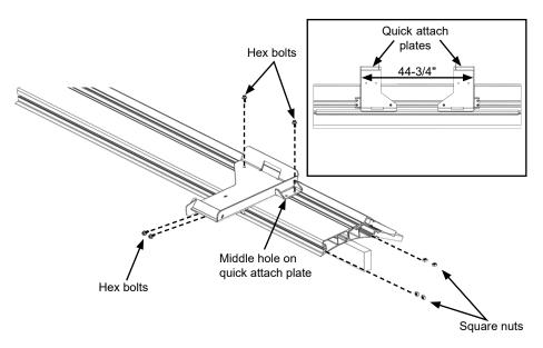
**NOTE:** One piece plows will use (2) 3/8" x 1" self-threading flange bolts on the top and (3) 3/8" x 3-1/4" hex bolts, washers and nylock flange nuts in the back.
