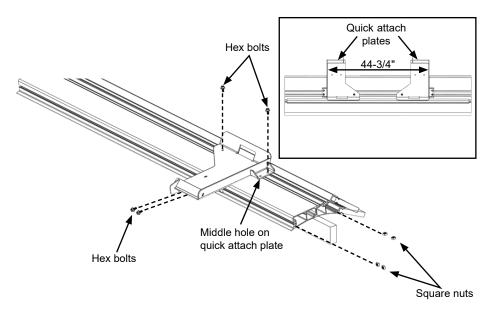
K. Use quick attach plates as template to drill 5/16" holes through back layer of aluminum at each factory marked location.
