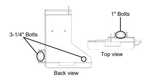
K. Use quick attach plates as template to drill 21/64" holes through back layer of aluminum at each factory marked location.
