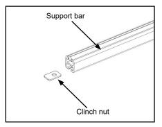
G. Adjust accessory bars as needed to place support bar on mounting plates, then insert serrated flange bolts through mounting plates into clinch nut in support bar. Leave loose for now.
