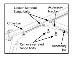
B. Remove accessory bar, then insert (2) additional mounting brackets into bottom channel of accessory bar.
