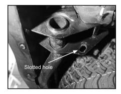
**NOTE:** Use proper orientation while installing brackets.
