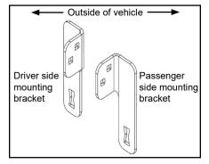
B. Insert carriage bolts into mounting bracket and through slotted hole. Secure with nylock flange nuts.
