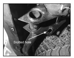
**NOTE:** Use proper orientation while installing brackets.
