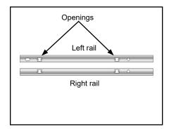
C. Align holes in rail over OEM rack system hooks, lift rail and route knots in cord through opening in rail, then turn (2) 3/8" x 3/4" hex bolts into threaded bracket and fully tighten.
