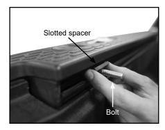
D. Place shim on bolt, gently lift up on bed cap and insert into OEM tonneau track.
