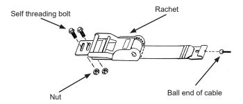
**NOTE:** Cable routing should appear as shown.
