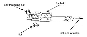
**NOTE:** Cable routing should appear as shown.
