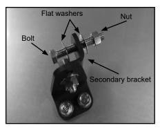
D. Thread nylock nut on hex bolt and place flat washer on bolt. Place lower pivot arm on hex bolt and secure with flat washer and nylock nut.
