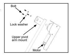
C. Lift motor and arm up to cartridge on roll tube then square motor with roll tube.
