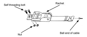
**NOTE:** Cable routing should appear as shown.
