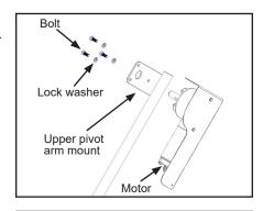
C. Lift motor and arm up to cartridge on roll tube then square motor with roll tube.
