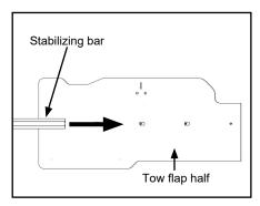
E. Insert Allen button head bolt through tow flap half into end cap assembly in stabilizing bar.
