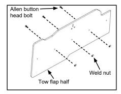
B. Insert weld nut into end cap aligning bolt holes.
