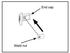
C. Insert end cap assembly into stabilizing bar.
