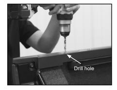
E. Place rail on box. Align rear hole in rail with drilled hole in bed cap.
