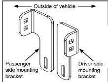
B. Insert carriage bolts into mounting bracket and through slotted hole. Secure with nylock flange nuts until snug, not completely tight.
