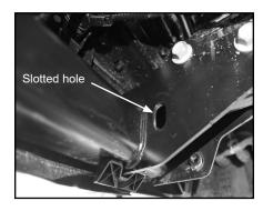
**NOTE:** Use proper orientation while installing brackets.
