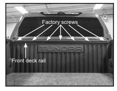
B. Replace factory screws once deck rail is removed.
