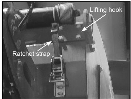
B. Install (2) Allen button head bolts where lifting hook was interfering with ratchet strap. Install (6) factory bolts at remaining locations.
