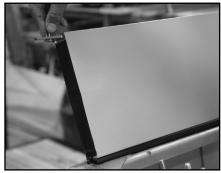
C. Align bolts on side extension with factory holes, then adjust side extension flush with outside edge of front extension. Secure with flat washers, lock washers and nuts, leaving finger tight.
