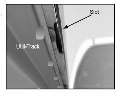
C. Loosen clamps and slide into slot in box rail, secure with nut.
