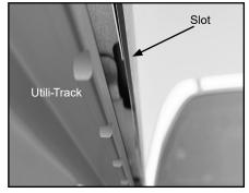
D. Loosen clamps and slide into slot in box rail, secure with nut.
