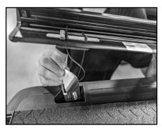
E. Align holes in pocket bracket and pocket brace, pull cord tight and place on bed rail.
