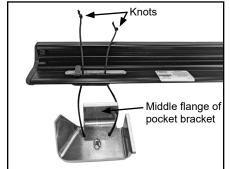
D. Lift utility rail and insert pocket bracket into stake pocket.
