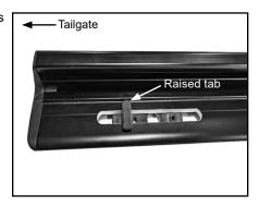
C. Position middle flange of pocket bracket to face outwards. Loop cord around extended threads on pocket bracket and through pocket brace, then tie knots at top of cord.
