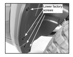
B. Install mud flaps with (4) factory screws through 2<sup>nd</sup>, 4<sup>th</sup>, 6<sup>th</sup>, and 8<sup>th</sup> slotted holes into newly free holes in wheel well. Leave screws loose for now.
