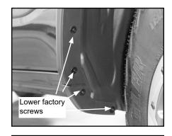
B. Install mud flaps with (4) factory screws through 1<sup>st</sup>, 3<sup>rd</sup>, 5<sup>th</sup>, and 7<sup>th</sup> slotted holes into newly free holes in wheel well. Leave screws loose for now.
