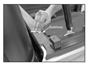
**NOTE:** Bulkhead depth may vary. Locate narrowest point to align bulkhead seal during application.
