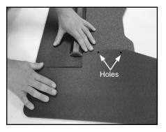
B. Drill (2) holes with 3/8" drill bit.
