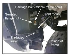
**NOTE:** For Mojave remote reservoir shock front mounts, use factory bolts and provided nylock flange nuts to secure with rachet and 10 mm socket. Fully tighten.
