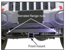
**NOTE:** 7/16" x 1-1/2" carriage bolt and hexhead cap screw placement may be reversed on some models, depending on threaded insert placement. Hex-head cap screw goes into threaded insert
