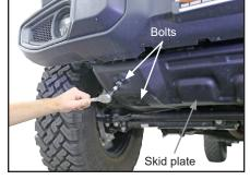
D. On one side, remove (2) inside skid plate bracket bolts with ratchet and 13 mm socket.
