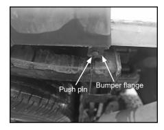
B. Place mounting bracket on top of bumper flange. Align hole in mounting bracket with hole in bumper flange.
