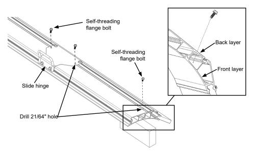
L. Torque (12) slide hinge bolts to 31 ft-lbs.
