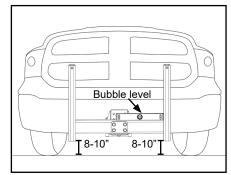
E. Check push frame for vertical plumb.
