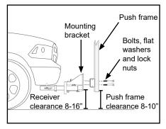
**NOTE:** In some cases, clearance under receiver may be less than 8". If so, plow will still operate properly, but ground clearance will be limited. Use care on uneven surfaces.
