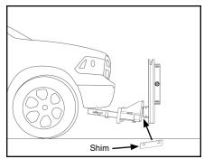
H. When shimming is complete, secure (4) 1/2" x 4" hex bolts with (8) flat washers and (4) lock nuts. Torque (4) nuts to 90 ft-lbs.
