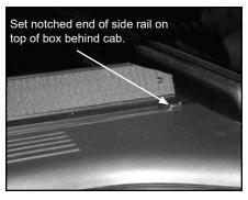
C. Start with clamp at front of box and work toward tailgate. Adjust clamps up or down until side rail is level after clamps have been tightened.
