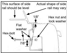
D. Lower side rail at rear until it is aligned 1/8" above box at center clamp location. After center clamp is tight, raise rear of side rail to correct height and position based on standard instructions and tighten rear clamp. Repeat Step 1 to install side rail on opposite side.
