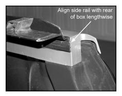
D. Move to second pre-punched hole in side rail. Align side rail with top of box and drill 1/8" hole. Then turn metal fastener in and tighten to 35 in-lbs. Repeat this procedure for 3rd hole from front of box.
