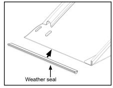
D. Peel protective backing then adhere seals to each side of end cap.
