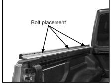
I. Tighten (3) bolts until flush, then torque to 85 in-lbs.
