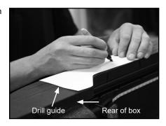
C. Drill 5/16" hole through bed cap and metal.
