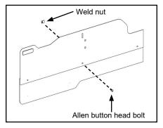
C. Insert weld nut into end cap aligning bolt holes.
