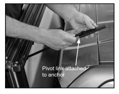
B. With anchor's post toward cover, test placement on top of cab in flat area between ribs. Ensure pivot link is flat against anchor's post, then mark location. Repeat for opposite side.
