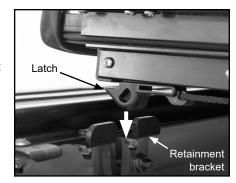
C. With cover in horizontal position, center on side rails, then slide front tabs fully under side rails and torque to 20 ft-lbs.
