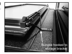
G. Release final latch and carefully tilt cover into storage bracket grooves for vertical position, then secure safety straps to side rails.
