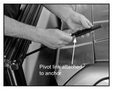
I. With anchor's post toward cover, test placement on top of cab in flat area between ribs, then mark location. Repeat for opposite side.
