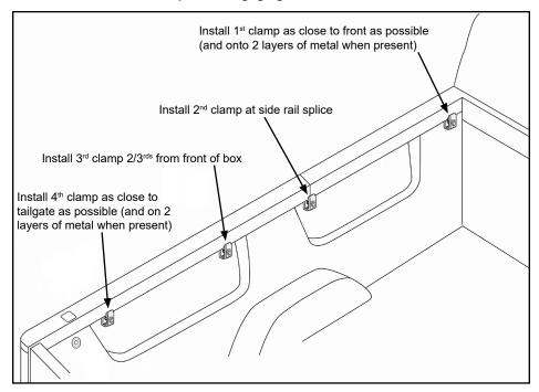
**NOTE:** For trucks with electric tailgates, typically side rail must be installed slightly higher to eliminate interference.
