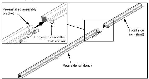
D. Attach short side rail (front) to assembly bracket with previously removed 1/4" x 3/4" carriage bolt and 1/4" nylock hex nut. Align side rails then tighten with 7/16" wrench.
