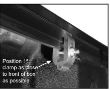
**NOTE:** Images below illustrate clamping options. **Option A** depicts standard clamping orientation lower on the side rail. **Option B** depicts alternate clamping orientation with half of clamp assembly rotated 180° to provide better grip at top of side rail.
