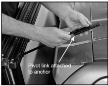
H. With anchor's post toward cover, test placement on top of cab in flat area between ribs. Ensure pivot link is flat against anchor's post, then mark location. Repeat for opposite side.
