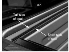
B. Starting at one end, peel protective backing as you go. Align and adhere seal against front of side rail and inside edge of box to opposite corner and cut to length.
