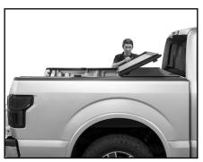
C. Always ensure hooks and latches fully engage side rails. Close tailgate.
