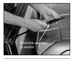
H. With anchor's post toward cover, test placement on top of cab in flat area between ribs. Ensure pivot link is flat against anchor's post, then mark location. Repeat for opposite side.
