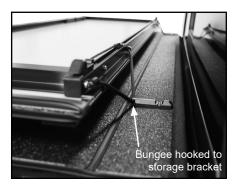
F. Release final latch and carefully tilt cover into storage bracket grooves for vertical position, then secure safety straps to side rails.
