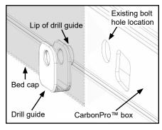
D. Start at front of box, use square hole to slide u-nut on CarbonPro™ box until extended threads align with existing bolt hole location.
