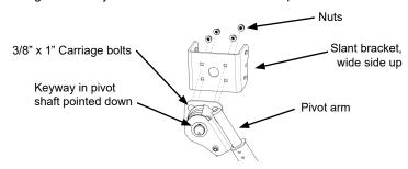
B. Bolt pivot arm with slant bracket to pivot mount using (3) 3/8" x 1" stainless steel carriage bolts, flat washers, lock washers and nuts and (3) 3/8" x 1-1/2" stainless steel carriage bolts, flat washers, lock washers and nuts. Leave bolts loose for now.
