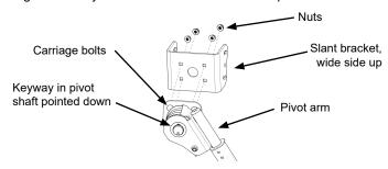
B. Bolt pivot arm with slant bracket to pivot mount using (3) 3/8" x 1" stainless steel carriage bolts, flat washers, lock washers and nuts and (3) 3/8" x 1-1/2" stainless steel carriage bolts, flat washers, lock washers and nuts. Leave bolts loose for now.
