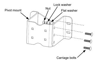
B. Slide (4) stainless steel square nuts into channels in mounting plate. Secure pivot mount to mounting plate using (4) 3/8" x 1" stainless steel bolts, lock washers and flat washers threaded into square nuts in channel. Center pivot mount on mounting plate and finger tighten all hardware.
