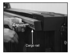
B. Cargo rail is still loosely attached to box with nylon anchors. Starting at front, pull cargo rail until anchors disengage and cargo rail is free from box. Installer should return cargo rail to owner.
