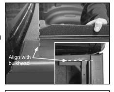
B. Adjust top of side rail until flush with top of box and hold with assistance of another person or a spring clamp.
