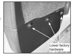
B. Install mud flaps with (3) 7 mm hex screws through 2<sup>nd</sup>, 3<sup>rd</sup> and 4<sup>th</sup> slotted holes into newly free holes in wheel well. Leave screws loose for now.
