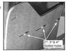
D. Install #10 x 1-1/4" self-drilling hex screw with washer at upper mounting hole.
