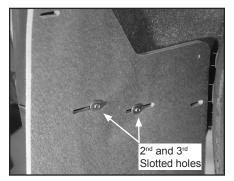
D. Install #10 x 1-1/4" self-drilling hex screws with washers at upper mounting hole and inside mounting hole. Secure inside mounting hole with nylon nut.
