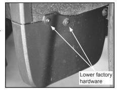
B. Install mud flaps with (2) 7 mm hex screws through 2<sup>nd</sup> and 3<sup>rd</sup> slotted holes into newly free holes in wheel well. Leave screws loose for now.
