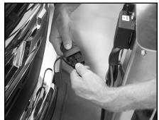
J. Attach quick connect plug on cab switch wire to winch plug and test system's operation with cab switch.
