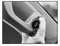
I. Attach quick connect plug on main power wire to winch plug and test system's operation with control box located on back of winch.
