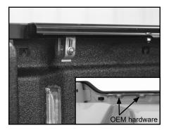
C. Continue to compress weather seal to inside lip of box and install fourth clamp between OEM hardware in box rail.
