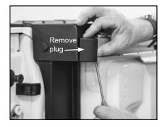
B. Assemble (3) brackets as shown, leave loose for now. Slide brackets into top channel of cargo rail and reinsert cargo rail plug.
