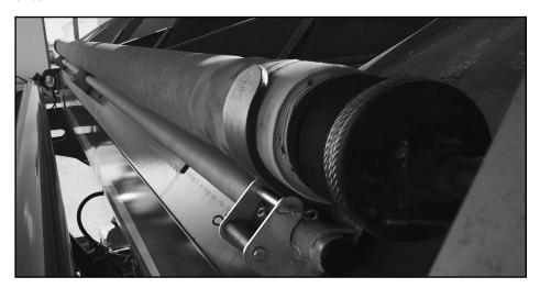
D. Z bracket and end caps located on front and rear of passenger side on top of box rail.
