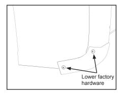
B. Install mud flaps with (2) 7 mm hex screws through 3<sup>rd</sup> and 5<sup>th</sup> slotted holes into newly free holes in wheel well. Leave screws loose for now.
