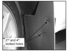
D. Install #10 x 1-1/4" self-drilling hex screws with washers at upper mounting hole and inside mounting hole.
