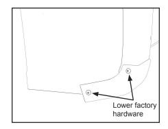
B. Install mud flaps with (2) 7 mm hex screws through 2<sup>nd</sup> and 4<sup>th</sup> slotted holes into newly free holes in wheel well. Leave screws loose for now.
