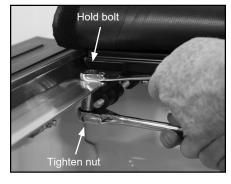
E. Center front bar between the two side rails.
