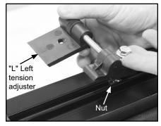
B. Turn 1-1/4" bolt with flat washer onto nut in front bar. Leave loose for now. Repeat for tension adjuster (marked "R") on passenger side of cover and leave bolt loose.
