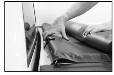
**NOTE:** Ensure alignment tabs are positioned perpendicular to cover and press against bulkhead.
