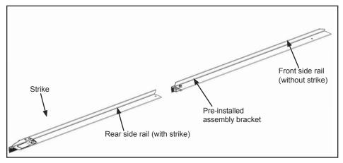
D. Attach rear side rail with strike to assembly bracket with flanged hex bolt and square nut, tighten with 1/2" wrench.
