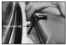
C. Slide left tension adjuster until it engages under side rail (see Step 3F). Push bar back and forth to line up holes. Do not turn adjustment wheel. Insert bolt from top then secure with nut from bottom.
