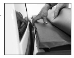
**NOTE:** Ensure alignment tabs are positioned perpendicular to cover and press against bulkhead.
