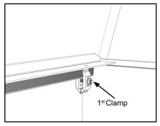
**NOTE:** Images below illustrate clamping options. **Option A** depicts standard clamping orientation lower on the rail. **Option B** depicts alternate clamping orientation with half of clamp assembly rotated 180° to provide better grip at top of rail.
