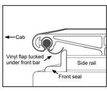
F. With the tension adjuster's support tab under the side rail, tighten bolt (left loose earlier) under front bar on each tension adjuster.
