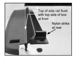
F. At front, adjust top of side rail until flush with top of box and hold with assistance of another person or a spring clamp.
