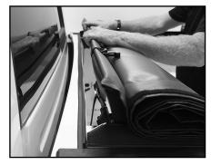
C. Slide left tension adjuster until it engages under side rail (see Step 5F). Push bar back and forth to line up holes. Do not turn adjustment wheel. Insert bolt from top then secure with washer and nut from bottom.
