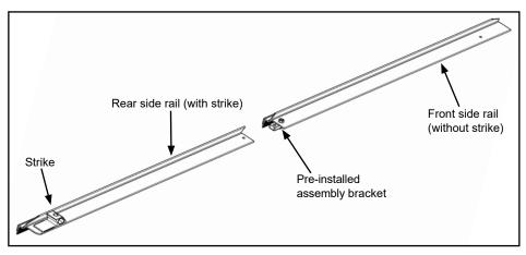
D. Attach rear side rail with strike to assembly bracket with flanged hex bolt and square nut, tighten with 1/2" wrench.
