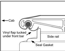
F. With the tension adjuster's support tab under the side rail, tighten bolt (left loose earlier) under front bar on each tension adjuster.
