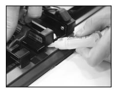
D. Secure channel with non-marring clamp and allow glue to dry (as directed by glue packaging).
