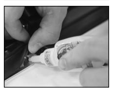
F. Center ridges in between both panels and hold hinge in place and allow glue to dry (as directed by glue packaging).
