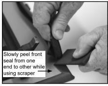
**NOTE:** In some cases, debris is left behind when removing the front seal. Patiently use included non-marring scraper or optional adhesive removal wheel to remove debris.
