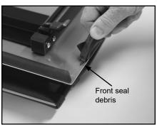
E. Use adhesive remover wipes to eliminate adhesive residue along the front of the cover.
