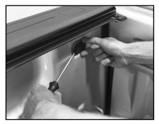
B. Under stake pocket hole, clean area with alcohol pad and apply adhesive protective strip. Save alcohol pad for later steps.
