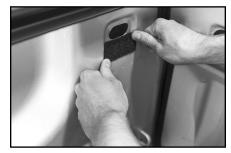
C. Insert long end of plate on front clamp assembly down into stake pocket hole and turn nut finger tight.
