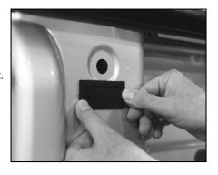
B. At top of rear stake pocket, lower back half of long clamp with fish wire and carriage bolt into pocket.
