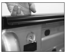
D. Place other half of clamp over bolt and turn nut finger tight.
