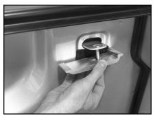
D. Ensure side rail is level and torque front clamp to 10 ft-lbs with 1/2" deep well socket and torque wrench.
