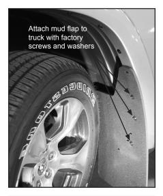
Attach with self-drilling screw and washer
