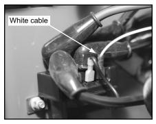
G. Attach black cable to connector on terminal block closest to outside of box.
